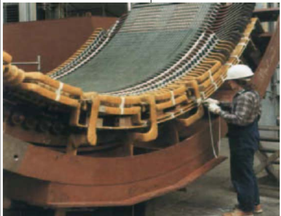
Fig.10 End winding reinforcement and circuit connections.
